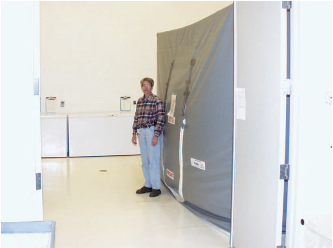
FIGURE 7. View of the quarantine and fumigation area at the Oklahoma Museum of Natural History, Norman, with the museum's registrar standing beside an inflatable CO 2 fumigation chamber and "fumigation" freezers in background. Photo by author.
